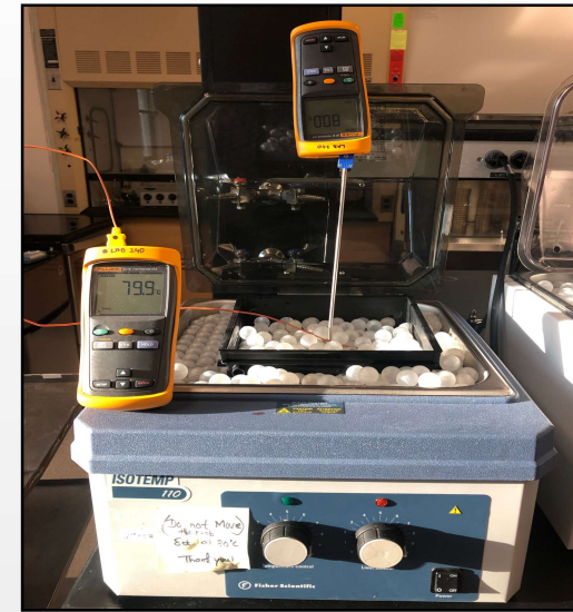
Thermocouples used for monitoring product and water temperature
