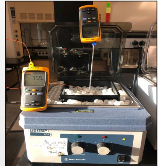
Thermocouples monitoring the product and water temperature
