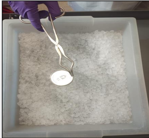
Transferring treated TDT discs to ice water bath
